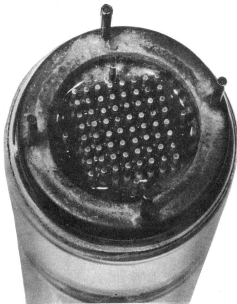
Figure 11. Electrical Matrixatron target assembly constructed at NEL.
